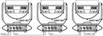
The communicate cable is 2-pin shielded cable  $75\Omega$
